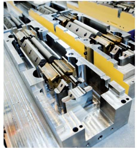
Magnets for the Swedish MAX IV synchrotron.
