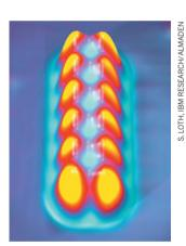
antiferromagnetic iron atoms in a regular pattern (pictured) on a copper nitride surface, and switched their magnetic states by applying a current of more than 7 millivolts to individual atoms using the tip of a scanning tunnelling microscope. From images taken with the microscope, the authors could distinguish two stable and distinct magnetic states of the atoms.
