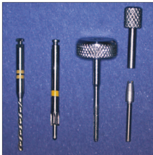
Fig. 5. K4 anchor post system consisting of from left to right post space drill (width reamer) and root facer (similar to that of the Radix anchor system), a tapping device (thread cutter) which cuts the counter tap into the walls of the post hole, and the threaded post together with the driver above.
