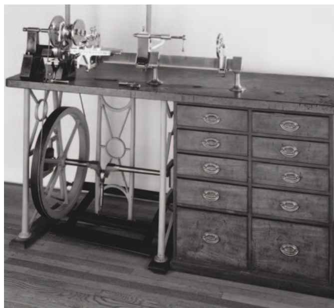
Fig. 7 24 An 1810 Maudslay lathe with tool drawers. Henry Maudslay (1771–1831) started his own lathe-making business in 1797. By kind permission, the Science Museum.
