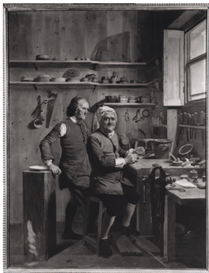
Fig. 6 Johan Zoffany, John Cuff and his assistant. 1772. This charming painting shows Cuff at his lathe beneath a sash window, with a pillar vice to his right. His assistant leans on a swaging block. The Royal Collection © 2004, Her Majesty Queen Elizabeth II.
