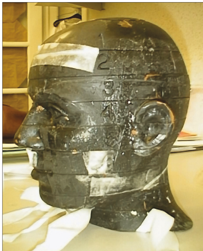
Fig. 2 The Rando® phantom head consists of a human skull surrounded and filled with tissue equivalent material. The slices allow positioning of dosimeters in pre-cut holes
