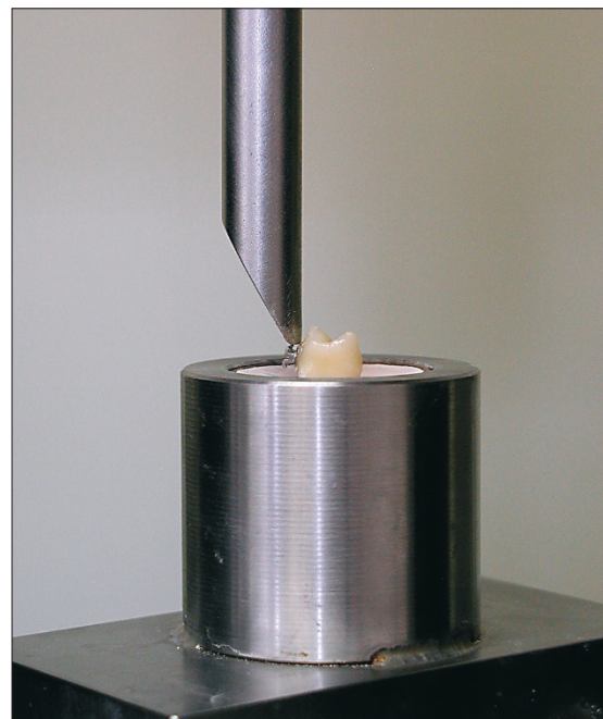
Fig. 1 Mounted specimen and testing jig
