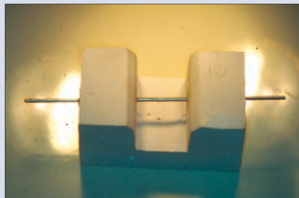
Fig. 2 Device used in order to control the alignment of the two pieces of wire
