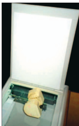
Fig. 5 Models on 3D scanner
