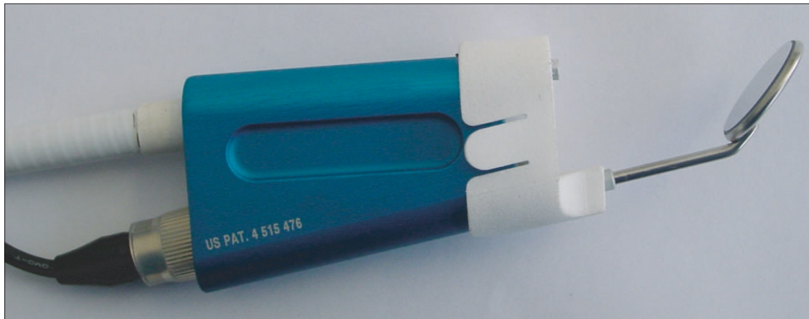
Figure 1. The QLF handpiece is comprised of a small CCD camera and a dental mirror. The light is carried in a fluid-filled cable to the camera from the distant source.
