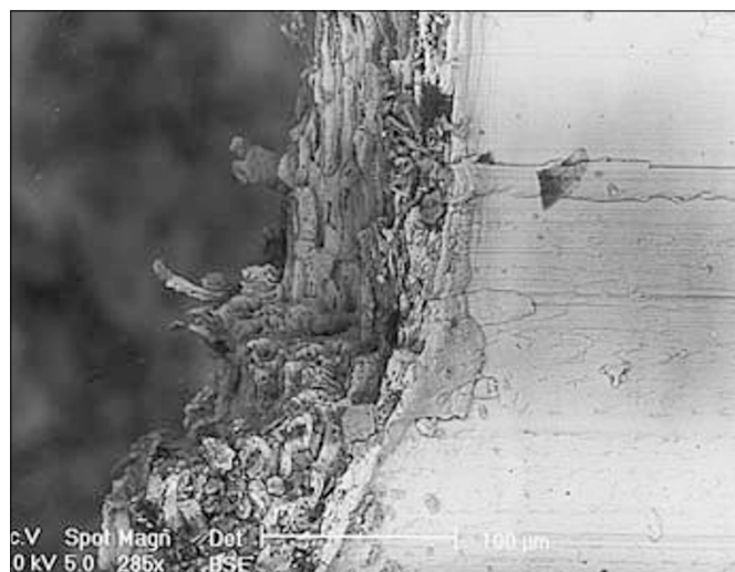
Figure 3. Scanning electron microscopy (Back Scattered Electron image) through the cannula of a dental syringe used in routine dental practice showing extensive biofilm formation. Measuring bar represents 100µm.
