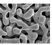
unknown, the authors think that the adsorbed anions may be slowing down the movement of inherent defects at the surface of the nanoporous gold, enhancing the material's strength. They anticipate the development of a material that can be made ductile during moulding or fabrication, and tuned to the strong state when desired.
