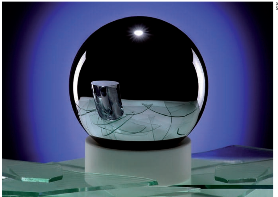
The silicon-28 sphere is the latest contender in a long weighting game.
