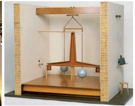
A model of Henry Cavendish’s torsion balance (above) and its latest successor, a laser interferometer.
