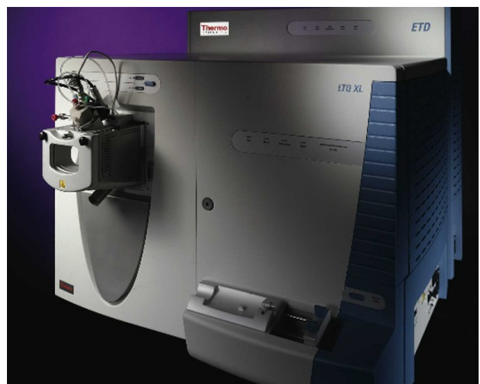
Thermo Fisher Scientific's Proteome Discoverer software (left) along with its L70 Orbitrap XL ETD system are being used to analyse histone modifications.
