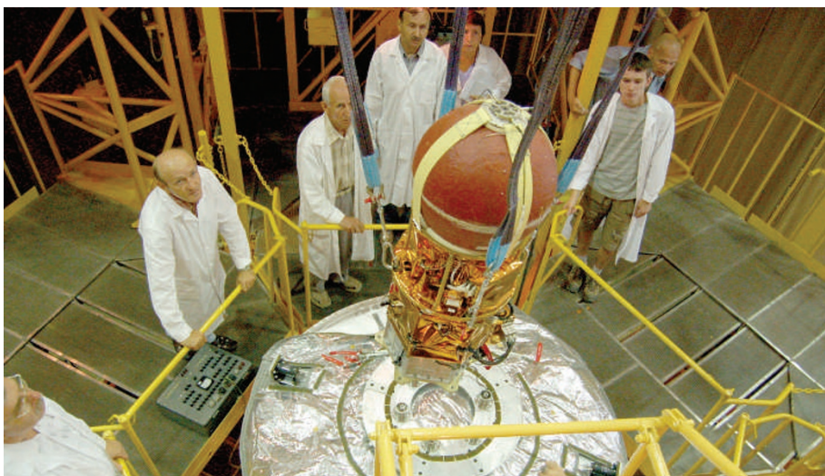
YES2, a 6-kilogram capsule (pictured), was hung from a satellite by a tether before falling to Earth.
