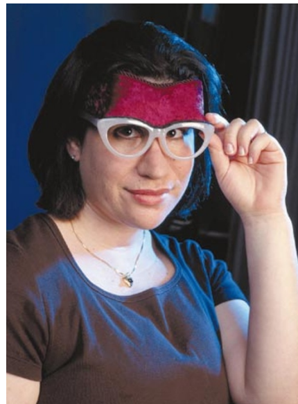
Curious or confused? These spectacles, developed at Media Lab, can help monitor the emotions revealed by a furrowed brow.
