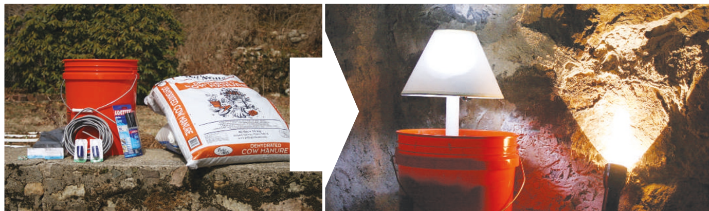
The power of mud: soil bacteria free up electrons as they respire. When used to induce a current between electrodes, these can light up a lamp.
