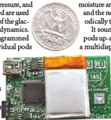
Watchful eyes: tiny computers called motes may one day be in everything.
