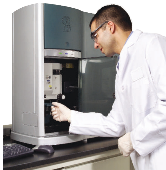
The Trilogy Single Molecule Analyzer can be used for miRNA detection.
