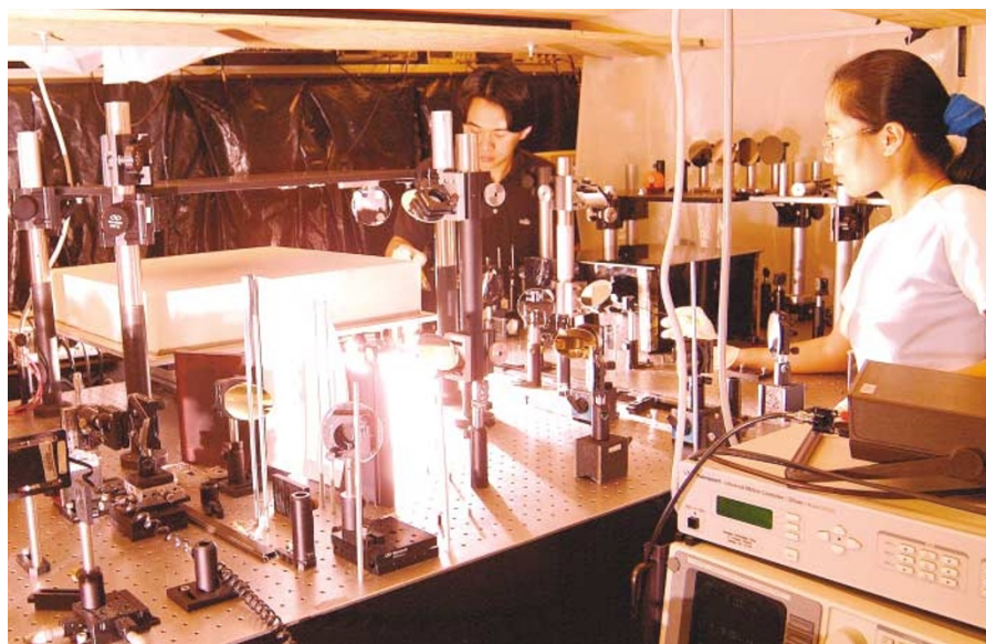
What lies within: researchers have successfully used terahertz radiation to spot internal defects in insulating foam (inset) for the space shuttle.
