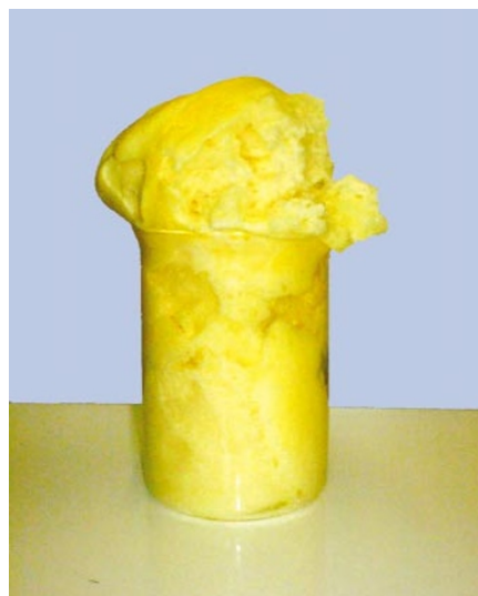
Figure 1 Light fantastic: up to 3 litres of a low-density, bright yellow vanadium oxide foam are formed when 1 g of V_2O_5 reacts with hydrogen peroxide in the presence of hexadecylamine.
