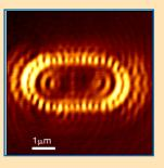
which can also be used to move loose atoms around on a metallic surface and position them into a closed loop. The electrons confined within these corrals interfere with one another and produce beautiful patterns, which the STM images make manifest. These experiments have been highly instructive for illustrating the quantum-mechanical principle that electrons can behave as waves.
