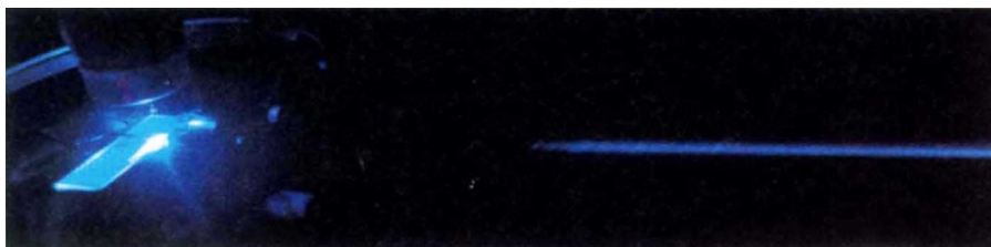
Blue-chip research. Gallium-nitride-based blue laser diodes such as this may soon be in our CD players and multimedia machines. (Picture courtesy of Nichia Chemical Industries Ltd.)
