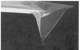
Tipped off - a carbon nanotube (some 10 nm in diameter and 100 nm long) stuck on the end of a conventional silicon probe used in scanning force microscopy. The probe and its associated cantilever arm are made of silicon. The nanotube tip is attached by coating the larger probe with glue and then bringing it in contact with a bundle of nanotubes; on pulling the probe away, a single tube can be left stuck on the probe's end.
