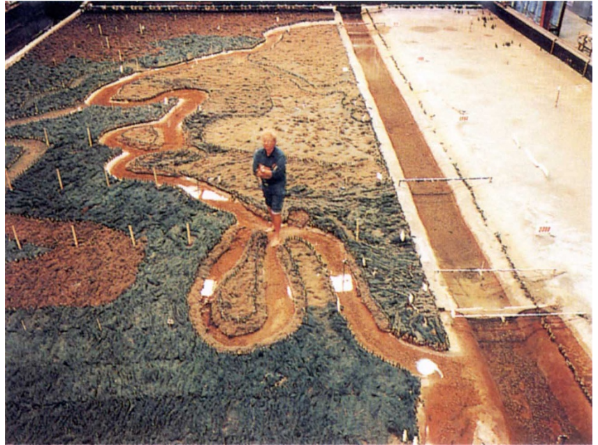
MODEL of the Kissimmee River, South Florida, as used by engineers and ecologists at the University of California at Berkeley to simulate restoration of this river-floodplain ecosystem. From Humanature , a collection of evocative photographs reflecting our relationship with nature. University of Texas Press, $60 (hbk), $29.95 (pbk).
