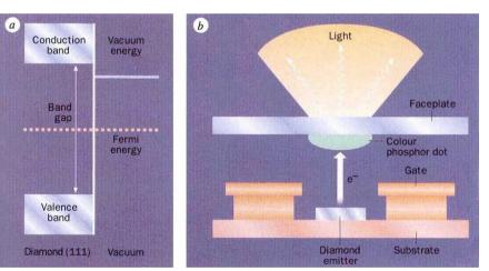
fact that the carriers do not move through the solid state but through a vacuum. In addition, cold cathodes could provide electron emitters for phosphorescent display devices (part b in the figure), whose fabrication requires only simple lithographic procedures. Several devices of this kind have now been demonstrated.
