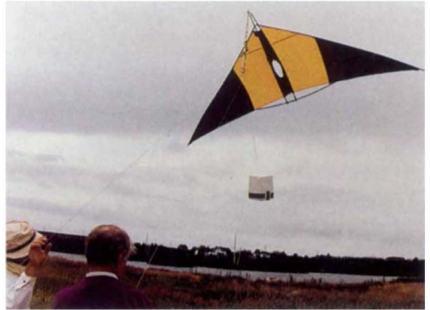
Photograph of the WindTRAM connected to the kite tether. The WindTRAM is designed to carry the sonde payloads up and down the tether while the kite remains aloft.
