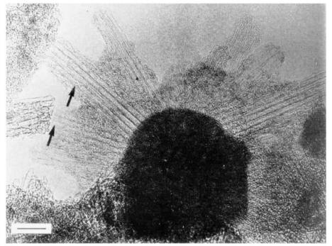
High-resolution transmission electron microscope image of bundles of short predominantly single-layer carbon tubes encapsulating an amorphous core of Gd<sub>x</sub>C<sub>y</sub>. Scale bar, 10 nm. Arrows, possible multi-wall tubes. The microscope is a Phillips CM20 ultra-high resolution TEM.
