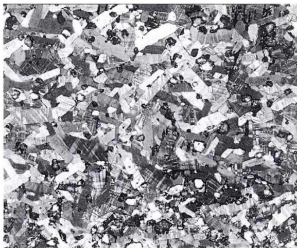
Polarized light micrograph of the high- T_c superconducting ceramic yttrium-barium-copper-oxide YBa_2Cu_3O_{6.9} (magnification \times \sim 90 ).
