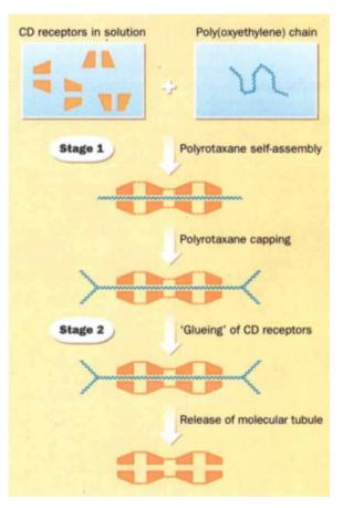
Building designer polymer tubes out of cyclodextrin units. In stage 1, dotted lines represent hydrogen bonds; in stage 2, these are replaced by covalent bonds between adjacent CDs.
