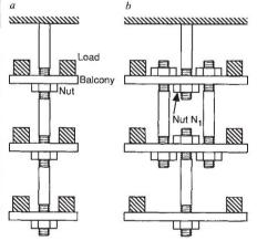
load on nut N1, causing three hotel balconies to fall when N1 split. Note that b distributes the load over seven nuts instead of the three nuts of a. This structural failure, as in the case of the springs and electrical circuits described by Cohen and Horowitz, falls into the category of series-to-parallel transformations.
