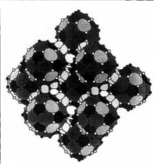
A fragment of the structure described in the text. Filled circles are C(1), shaded circles are C(2) and open circles are C(3). The lighter-shaded hexagons are parts of hexagonal prisms.
