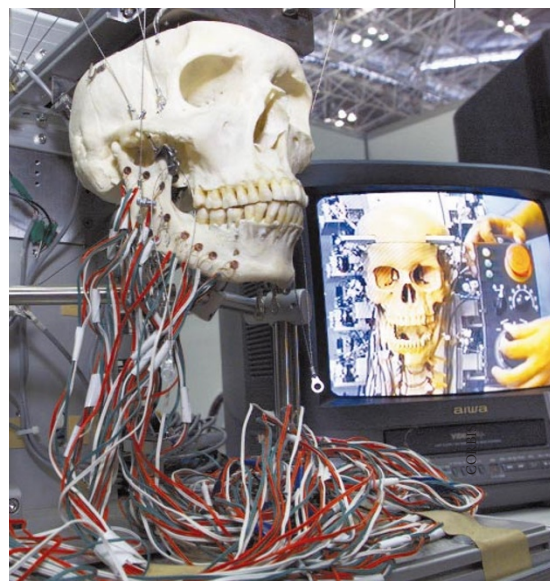
Profitable tool of the trade: a mastication robot developed by researchers at Waseda University.
