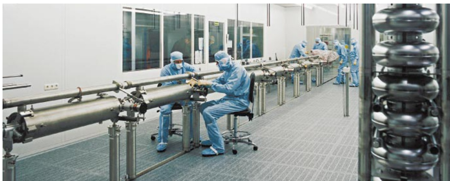
Linear thoughts: DESY staff assemble prototype accelerator parts for the proposed TESLA collider.
