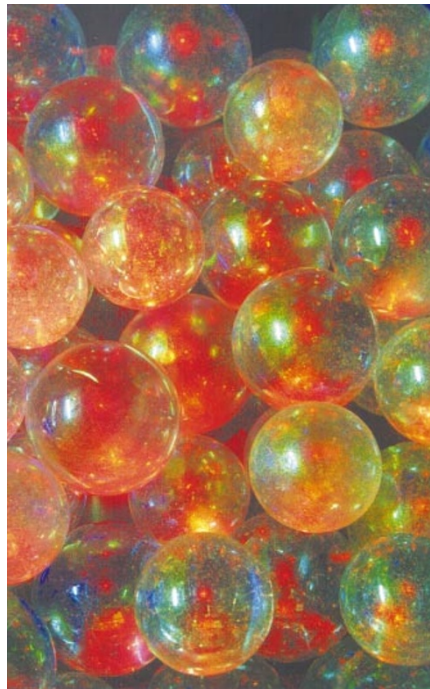
Figure 2 Model of an amplifying disordered material used to build a 'random laser'. Green light is multiply scattered by the spheres and charges the system, thereby enabling the amplification process. The red light is both multiply scattered and amplified. The combination of multiple scattering and amplification leads to random laser action. Miniature random lasers can be used as sources in optical devices, such as wave-guides or all-optical switches. Their tiny size also makes them suitable for marking documents or materials in a hidden way.
