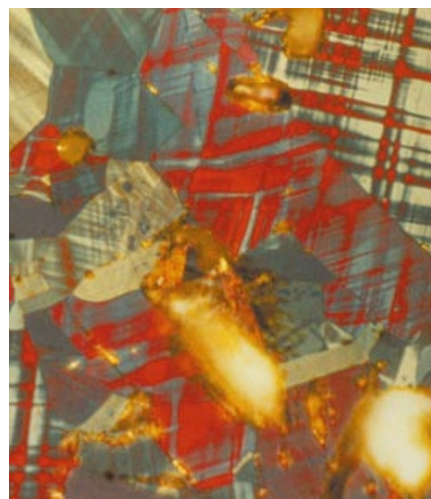
Coveted prize: polarized light micrograph of a YBCO high-temperature superconductor.
