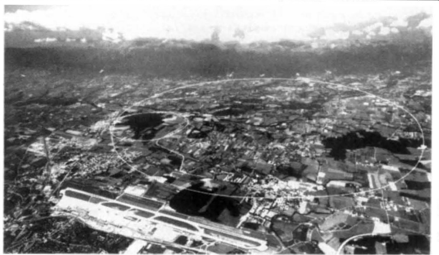
THE completion of the large electron-positron collider (LEP) was announced last week by CERN, the European laboratory for particle physics. The circular machine, housed in a 27-km-long tunnel between 50 and 150 m below the surface, accelerates electrons and positrons to a combined energy of 200 GeV. LEP's main purpose is to investigate the Z^0 particle, discovered at CERN, and although the Stanford linear collider recently made its first Z^0 ( Nature 338, 606; 20 April 1989), LEP has more than two times the beam energy of its rival and is expected to generate Z^0 's at a higher rate. LEP is the result of an eight-year project financed by the 14 member states comprising CERN. □
