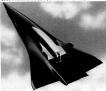
The plane, named after German aerospace pioneer Eugen Sänger (1905–1964), would consist of two reusable parts: a booster stage resembling a conventional jumbo- jet would bring a smaller craft piggyback to an altitude of 30 km. The smaller plane would then fly at five times the speed of sound to its destination. Sänger could be used for passenger transport on Earth or as a space shuttle.
