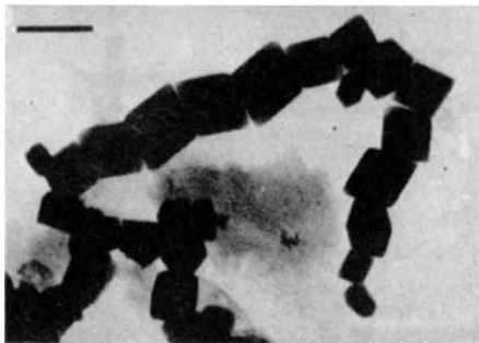
A chain of biogenic magnetite grains identified by Petersen et al. from deep-sea sediment cores. But not all magnetite is biogenic, Maher and Taylor show 1 . (Scale bar, 0.1 \mu\text{m} ; from ref. 8.)
