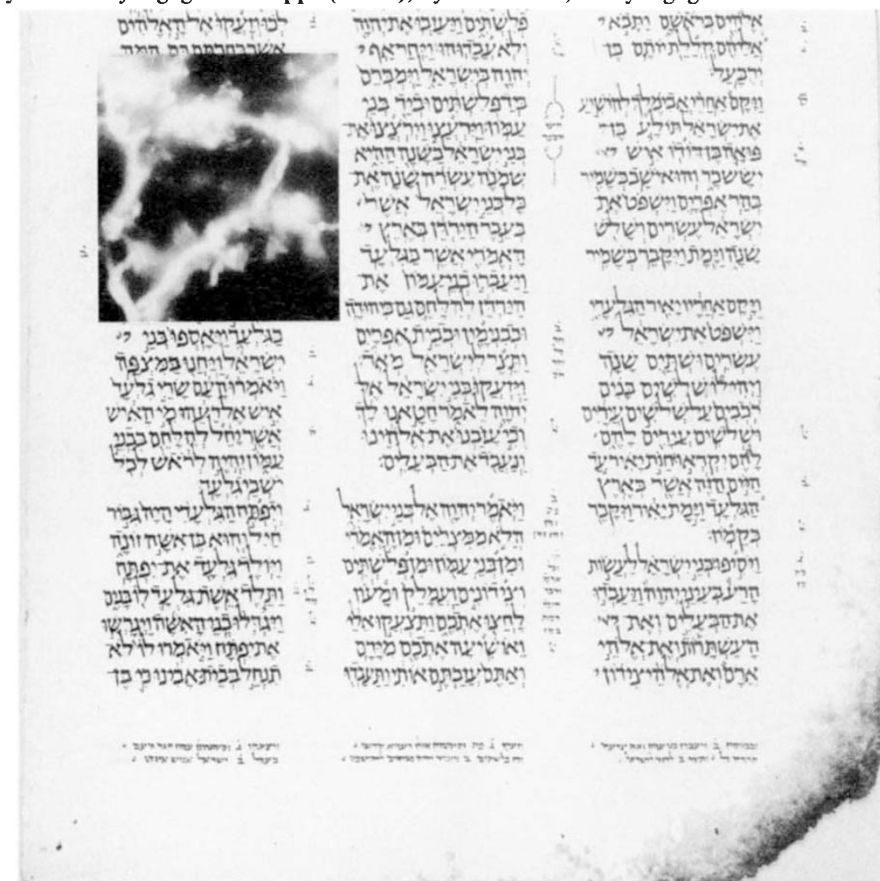
A page from the Codex showing typical discoloration and deterioration in the outer lower corner. Inset: fluorescence photomicrograph of fungus-like filaments in the damaged areas. Preparations mounted in the fluorescent fungal stain Cellufluor (Polysciences), KOH and glycerol. \times 600 .
