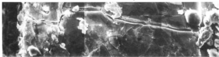
Cross section through a latex glove ( \times 1,700 ) with the exterior surface on the left.
