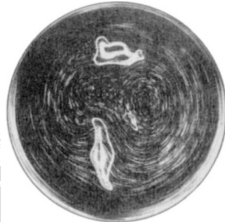
Horizontal streak pattern from the dish-pan experiment of Boyer and Chen. The solid white objects are the forms representing the Rockies, the Himalayas and Greenland. (From ref. 1.)
