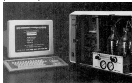
A DNA synthesizer that uses all chemistries.
