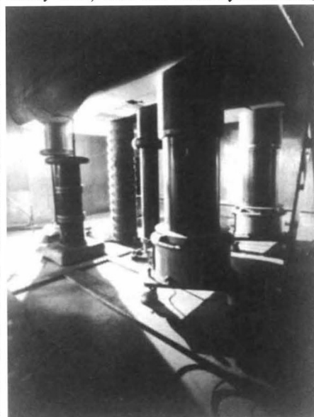
Isolation supports of Saturne's polarized particle source.
