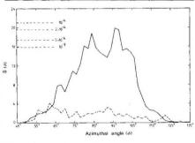
The azimuthal modulation of the plane containing the electron-positron pairs derived from 2,526 pulsed Vela  $\gamma$ -rays that materialize in the Cos-B spark chamber (solid curve). The dashed curve applies to 3,109 photons from the Cygnus region used as a comparison. *S* is the deviation function as defined in Caraveo *et al.* Overall chance occurrence probability levels are shown as derived from Monte-Carlo simulations.
