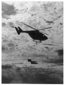
re-entry vehicle. The white twin-finned shuttle was released at 1,000 m from a helicopter flying at 200 km per h 5 km off the Akita coast of Japan.
