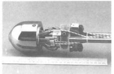
A REVIEW article on page 127 of this issue describes experiments that provide new optimism for the possibility of generating power from nuclear fusion. The picture above shows the target capsule used to hold the deuterium-tritium mixtures for muon-catalysed fusion experiments at the Los Alamos Meson Physics Facility in 1984. The target was electrically heated to 800 K and then cooled to 14 K with liquid helium. Up to 150 fusions per muon (average) were observed with this apparatus.
