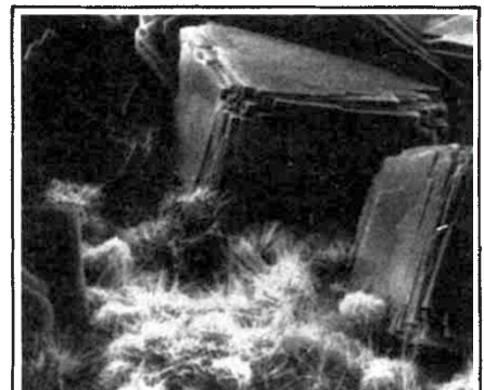
Scanning electron micrograph ( \times 975 ) of basalt glass after leaching in NaCl solution at 200°C for 30 days — a model for the stability of nuclear waste glasses. See page 252.
