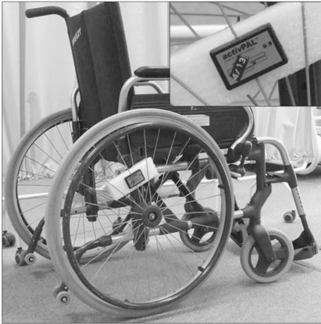
Figure 1 Demonstrating the attachment of an activPAL activity monitor to the wheel of a manual wheelchair. Inset: close-up of the activPAL activity monitor.
