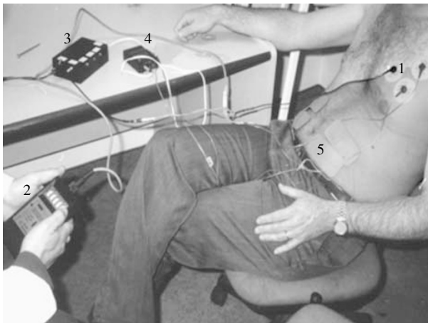
Figure 1 The EMG-activated FES system, demonstrated on a healthy person: Recording surface electrodes (1), the Omnistim IV stimulator (2), manually adjustable interface (3), the quick off muscle stimulator (4), and abdominal stimulating surface electrodes (5)
